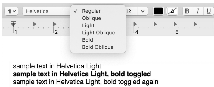
FIG. 11.2 Integrity violation example in TextEdit: bolding once (second line) turns the text from light to bold; bolding again (third line) leaves the text in regular, not light.
